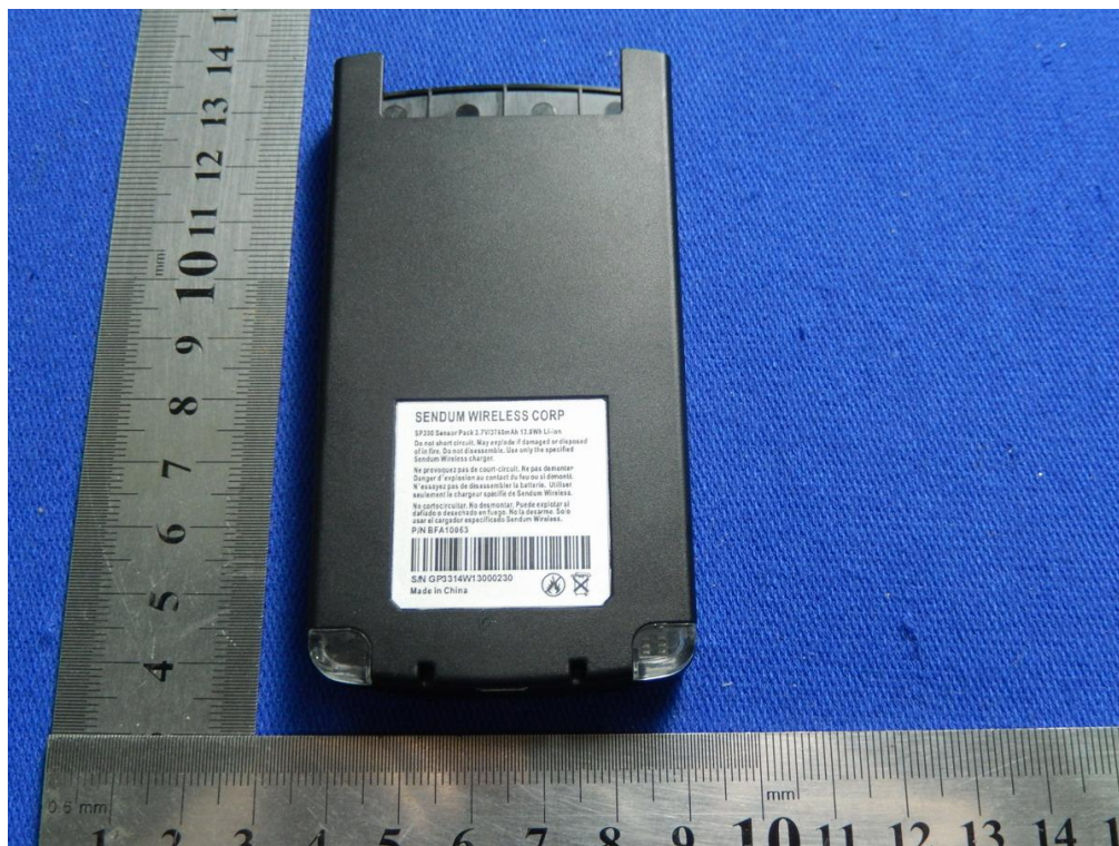
Battery (SP300 3,7V 3760mAh 13,9Wh)
