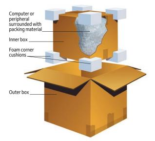
Since this type of packing material allows the packaged item to settle to the bottom of the box, it is important to use the overbox method of packaging. The inner box should be at least 10 cm (4") greater in length, width and height than the item you are shipping. This will allow for 5 cm (2") of space for all six sides. The outer box should be at least 15 cm (6") greater in length, width and height than the inner box. This will allow 8 cm (3") of space between the inner box and the outer box.
